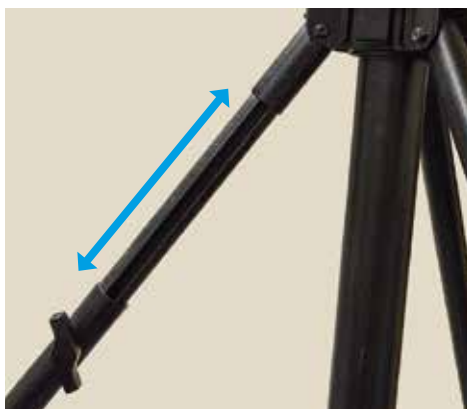
Extendable tripod leg for uneven slopes
